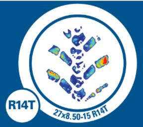
Inflation Pressure: 10 psi Tested Load: 723lbs Contact Area: 18.54 in<sup>2</sup> Footprint Area: 59.62 in<sup>2</sup> Ave Contact Pressure: 37.89 PSI Contact to Void Ratio: 31%
