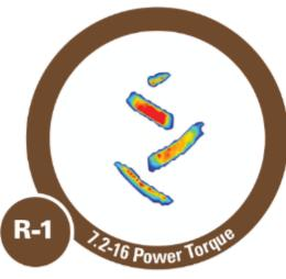
Inflation Pressure: 14 psi Tested Load: 723lbs Contact Area: 10.53 in<sup>2</sup> Footprint Area: 38.59 in<sup>2</sup> Ave Contact Pressure: 67.53 PSI Contact to Void Ratio: 27%
