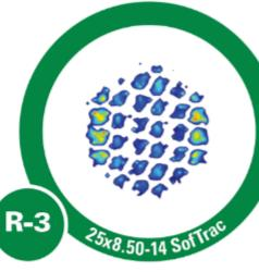
Inflation Pressure: 10 psi Tested Load: 723lbs Contact Area: 22.67 in<sup>2</sup> Footprint Area: 46.92 in<sup>2</sup> Ave Contact Pressure: 31.38 PSI Contact to Void Ratio: 48%
