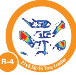
Inflation Pressure: 10 psi Tested Load: 723lbs Contact Area: 16.08 in<sup>2</sup> Footprint Area: 47.82 in<sup>2</sup> Ave Contact Pressure: 44.2 PSI Contact to Void Ratio: 34%
